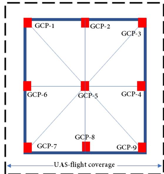
Figure 1. Ground Control Point (GCP) distribution
