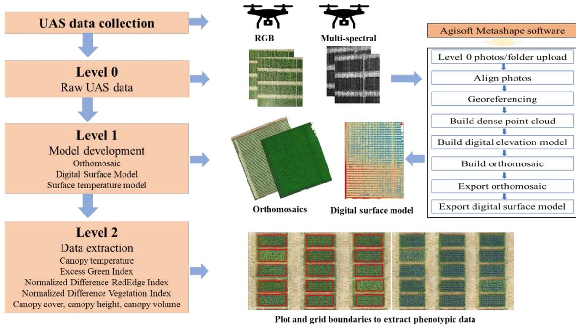
*Figure 6. Data processing pipeline*
